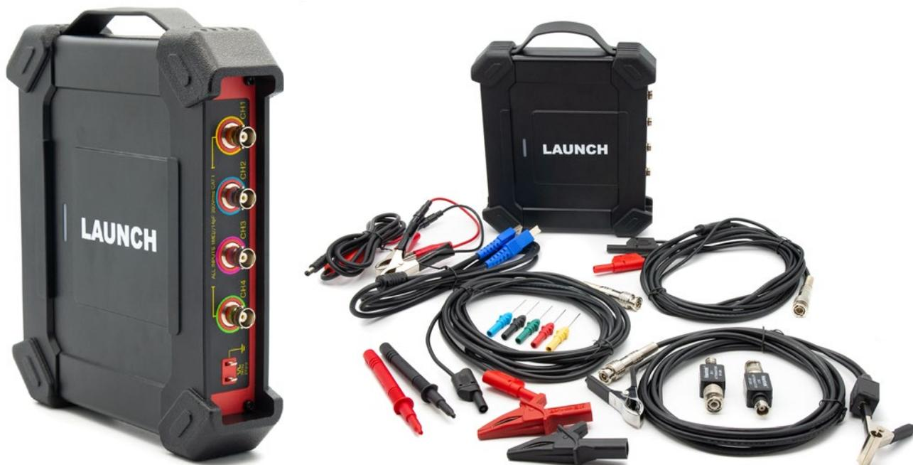
The X-431 02-1 Scopebox is a four-channel automotive oscilloscope designed for use with the Launch Euro Tab 2 & Euro Tab 3. The Scopebox is used with one of two apps on the diagnostic tool: scopebox & Ignition scope.
