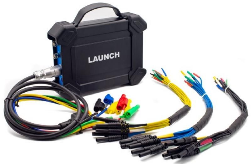
The Launch S2-2 Sensorbox has been specially developed to diagnose automotive actuator and sensor faults. It can simulate the sensor input signals to the vehicle electronic control systems, and the control system output signals to the actuators.
