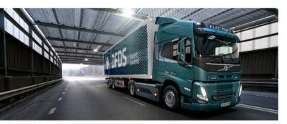
The largest available Volvo truck is the FM, designed for extra-urban use. With up to 44 tonnes GVW and 490kW of battery power, the FM enjoys similar charging times to its smaller stablemates, but a range of up to 300km when specified with the biggest batteries.
